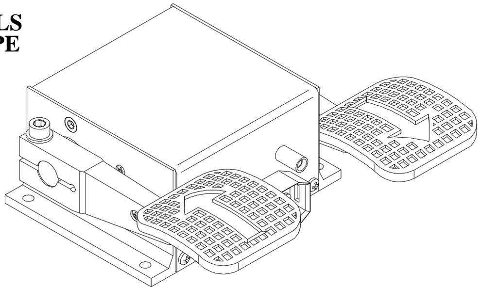
PR/1B and PE/2 foot pedals comply with all requirements concerning use in lift trucks and electric vehicles thanks to their compact size, simple assembling and electric connection through connector.
